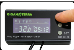
• Use the arrows to set the desired temperature. Confirm and go to the next setting by pressing SET.
