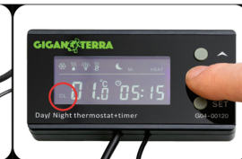
• Setting the temperature difference: DL flashes. Use the arrows to set the desired temperature. Confirm and go to the next setting by pressing SET.
