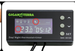
• Setting the night temperature SET and M flash.
