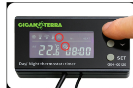
• Setting the start time of the day: C & S flash. Use the arrows to set the daytime temperature. Press SET to go to the minute setting. Confirm and go to the next setting by pressing SET.
