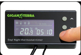
• 2nd step: Mode settings: HEAT / COOL. Keep pressing SET for 5s.
