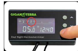
• Setting the temperature difference of the overheating alarm. M flashes. Use the arrows to set the desired temperature. Confirm and go to the next setting by pressing SET.
