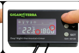
• 2nd setting the TIMER on the PLUG II: L2. Same as setting the L1 schedule. Confirm and go to the next setting by pressing SET.
