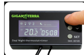
• Setting the maximum and minimum safety temperature. Press the ^ arrow for 5 seconds until 50 is displayed and set your desired maximum temperature. Confirm by pressing SET. Repeat the operation with the down arrow to set the minimum temperature.
