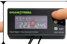
• Setting the current time: C flashes. Use the arrows to set the current time. Press SET to go to the minute setting. Confirm and go to the next setting by pressing SET.
