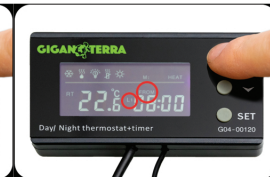
• 1st setting the TIMER on the SOCKET II: L1. Use the arrows to set the start time FROM flashes. Press SET to go to the minute setting. Press SET to switch to the end time setting in the same way, TO flashes. Confirm and go to the next setting by pressing SET.
