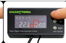
• 2nd setting the TIMER on the PLUG II: L2. Same as setting the L1 schedule. Confirm and go to the next setting by pressing SET.
