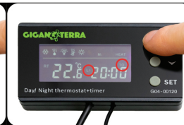
• 1st setting the TIMER on the SOCKET II: L1. Use the arrows to set the start time FROM flashes. Press SET to go to the minute setting. Press SET to switch to the end time setting in the same way, TO flashes. Confirm and go to the next setting by pressing SET.
